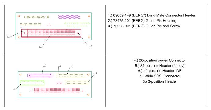
Figure 9-1: Peripheral Bay Board (Chassis Side) Layout
